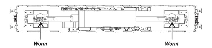
To expose drive worms and chassis for routine maintenance, simply pull the complete bogie assembly away from the chassis. The bogies are a 'pull-out' & 'push-in' fitting method. When refitting, ensure that the gear on top of the bogie tower meshes with the worm.
