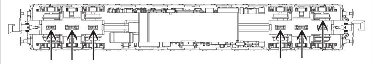
Normal oiling points into exposed gears without removing body
